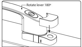
Rotate handle 180°. Align the bottom screw cover above & push down into place, until flat & fully engaged. Return the handle to its original position.
