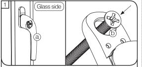
First check that you have the correct handle offset with the handle offset to the glass side, as shown above (a). Ensure the window and the espag handle are in the closed position. Insert a fixing screw into the top fixing hole (b). ProLinea Offset Espag Handle -Fitting Instructions
