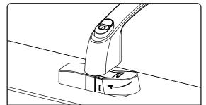
Press the button and rotate the handle counterclockwise by 90°. Slide the bottom screw cover into position at a 45° angle until flat & fully engaged. Return the handle to its original position.
