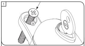
Ensure the window and the espag handle are in the closed position. Insert a fixing screw into the top fixing hole as shown above (a).
