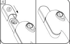
Close lever. Slide the screw cover (d) into position. Ensure cover sits flat, as shown
