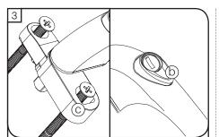
Press button (b) and rotate lever 90° to reveal bottom fixing hole (c) (caution window will open). Insert screw & carefully tighten.
