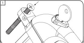
Ensure the window and the espag handle are in the closed position. Insert a fixing screw into the top fixing hole as shown above (a).
