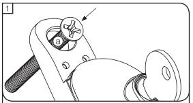
Ensure the window and the espag handle are in the closed position. Insert a fixing screw into the top fixing hole as shown above (a). ProLinea Espag Handle - Fitting Instructions
