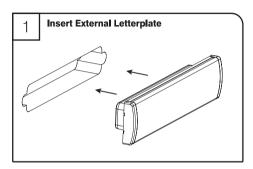
Begin by inserting the external half of the letterplate fully into the aperture on the external side of the door. Hold in place.
