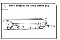
Fix the two halves together using supplied M5 fixing screws in the appropriate holes.
