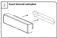
Fully insert the internal letterplate into the aperture on the internal side of the door.
