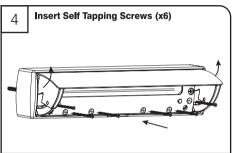
Now insert x6 appropriate length self tapping screws (not supplied) into the remaining holes to fix the letterplate securely to the door.
