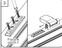
Fit the frame datum into the drilled 5 mm holes and screw in place. Take hinge and align the aperture with the frame datum and slide down into position.
