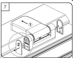
Release the sash cover (refer to step 1). Slide the cover in the direction shown (1). Using a flat blade screwdriver, release the cover caps (2).
