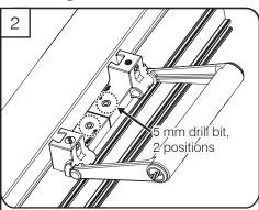
Using the Mila jig for alignment, pre-drill holes for frame datum using 5 mm drill bit.
