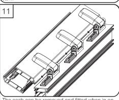
The sash can be removed and fitted when in an open position by lifting or lowering the sash assembly onto the frame datum.
