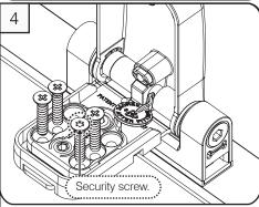
Lift cover and secure the sash part using 4x long screws (on a open outward door we recommend using security screws or a hinge protector).
