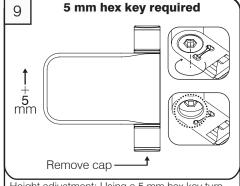
Height adjustment: Using a 5 mm hex key turn the screw up to lift the hinge by up to 5 mm.
