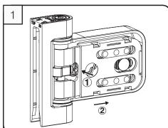
Using a flat blade screwdriver depress the latch beneath the sash part (1) to release the sash cover. Slide the cover in the direction shown (2) until fully disengaged.
