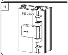
Close sash cover and slide back in the direction shown to engage the latch. Fit caps.
