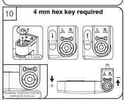
Compression adjustment: Push out hinge pin and turn to alter compression.
