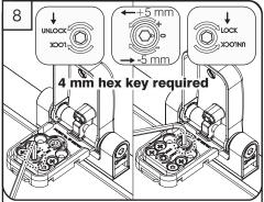
To adjust lateral position, first turn the unlock cam a 1/4 turn. Then use the adjustment cam to adjust up to 5 mm in either direction. Finally tighten lock cam.
