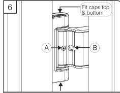
Open the door and locate position (B) (as shown above). Using the screw provided fit and tighten to secure the cover.
