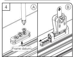
(A) Fit the frame datum into the drilled 5mm holes and screw in place. (B) Take hinge and align the aperture in the frame part and slide into position.
