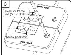
Align the jig using the underside pins then drill holes for the frame and sash part choosing the most suitable position for your door
