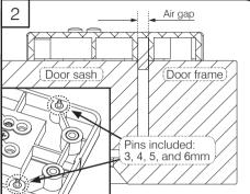
To correctly use the Mila jig, measure the air gap between the door sash and frame. Take the matching pin size and insert them into the underside of the jig, as shown above.
