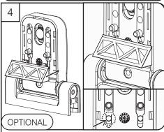
If required an optional profile dedicated packer can be fitted. Align pegs with holes in hinge and push to insert for positive fit.
