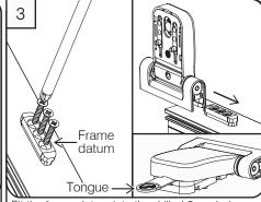
Fit the frame datum into the drilled 5mm holes and screw in place. Take hinge and align the aperture in the frame part and slide into position. Lift sash cover and remove tongue.
