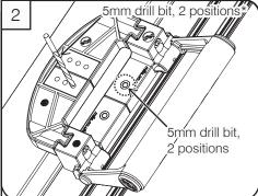
Using the Mila jig for alignment, drill holes for frame part and if fitting \*optional fixing pegs drill the sash part choosing the most suitable position for the pins on the profile.
