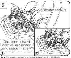
(1) Secure using 4x long screws & 2x short screws. Or (2) Use 4x long screws & 2x supplied fixing pegs. Close cover.
