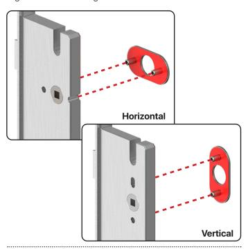
**4.** Insert the spindle & position the handle, then insert & tighten the screws ensuring they engage with the fixing plate (when fitting horizontally, angle the lever to fit the second screw). If required, add surface fixings in the spare screw positions, taking care not to hit the gearbox.
