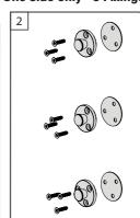
Using the screws provided, screw 'fitting A' to the 3 positions where you have marked, one on the top marking one on the middle and one on the bottom. make sure it is secure.
