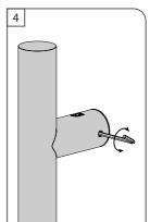
Tighten the grub screws at the top, middle and bottom fixing the handle to 'Fitting A'.
