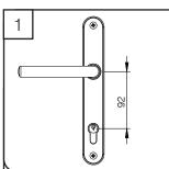
The measurement from the centre of the locking lever to the centre of the keyhole known as the PZ distance - the PZ distance of this handle is 92mm.
