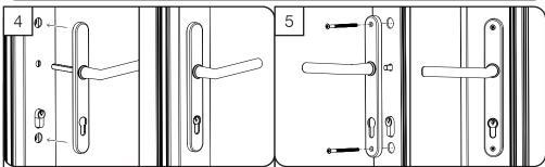
Insert correct length of spindle (supplied) into the external lever. Slide the spindle through the lock mechanism from the external side of the door. The external backplate should fit up against the profile clearing the cylinder lock.
