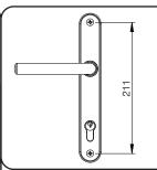
The distance between the centre of the top screw and the centre of the bottom screw - this distance on this handle is 211mm.
