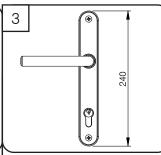
The length of the handle backplate, top to bottom - this handle backplate is 240mm long.
