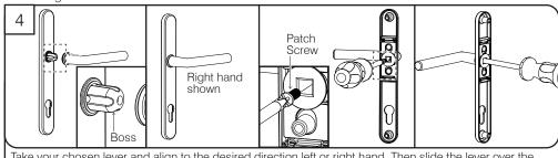
Take your chosen lever and align to the desired direction left or right hand. Then slide the lever over the boss. While holding the lever by hand apply pressure to ENSURE THE LEVER IS FULLY UP AGAINST THE BACKPLATE. Take the patch screw (supplied) & insert the screw through the back of the boss into the lever. Tighten using a PH2 screw driver. IMPORTANT: The patch screw must be fully tighten to ensure the lever is fully secured. The screw will NOT be able to be adjusted after a 1 HOUR period.
