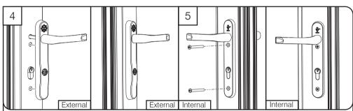
Insert correct length of spindle (supplied) into the external lever. Slide the spindle through the lock mechanism from the external side of the door. The backplate should fit up against the sash covering the cylinder lock. On the internal side of the door slide the backplate onto the spindle & up to the sash. Select the correct length screws (supplied) & insert through fixing holes & screw together taking care not to over tighten.
