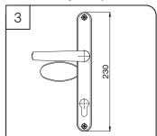
The length of the handle backplate, top to bottom - this handle backplate is 230mm long.
