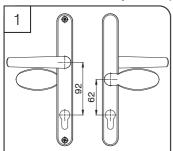
The measurement from the centre of the lever or pad to the centre of the keyhole, is known as the PZ distance. On this handle it's 62mm on the external side and 92mm on the internal
