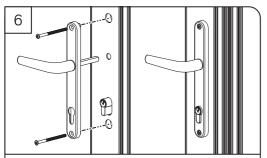
Slide the internal backplate onto the spindle and up to the internal profile. Select the correct length screws (supplied). Insert both screws and screw together taking care not to over tighten.
