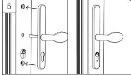
Insert correct length of spindle (supplied) into the external lever. Slide the spindle through the lock mechanism from the external side of the door. The external backplate should fit up against the profile clearing the cylinder lock.
