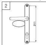
The distance between the centre of the top screw and the centre of the bottom screw - this distance on this handle is 211mm.
