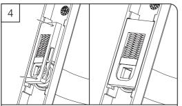
For non-sprung door locks both handles will require the supplied spring cassette to be fitted. As shown above, insert the spring cassette at an angle and then push firmly until located.
