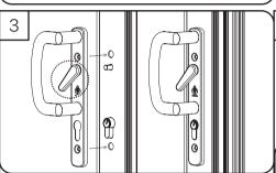
On the internal door side check that the lever is set as shown above. Then push the backplate onto the exposed spindle until the handle is flush against the door frame.
