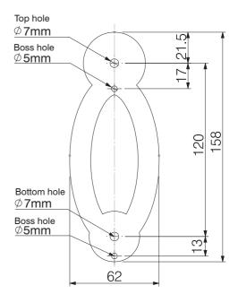
**6.** Mark the bolts and remove them to cut the excess off. Double check the depth of the door allowing for the bolts to go through And the nuts to screw onto after cutting. Reposition the door knocker and tighten up the nuts using a small spanner.
